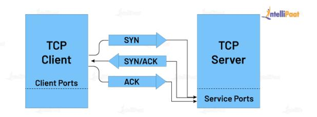
Step 1: The client makes a connection with the server with SYN.
